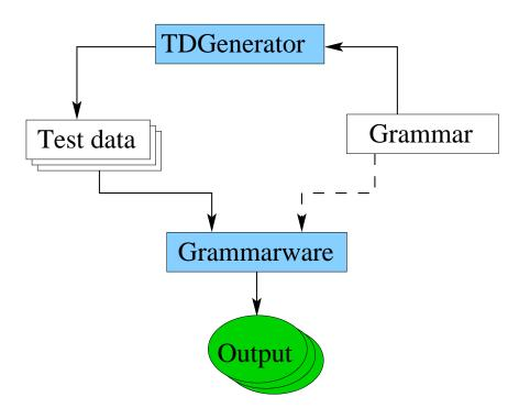
Grammar-based testing tool generates terms in a combinatorial way.
